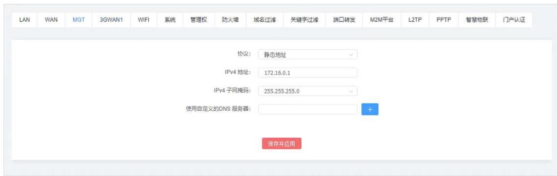
This screenshot shows the same MGT port configuration page as above, but with specific values entered: the IPv4 address is now 172.16.0.1 and the subnet mask is 255.255.255.0. The other fields and the "Save and Apply" button remain the same.
